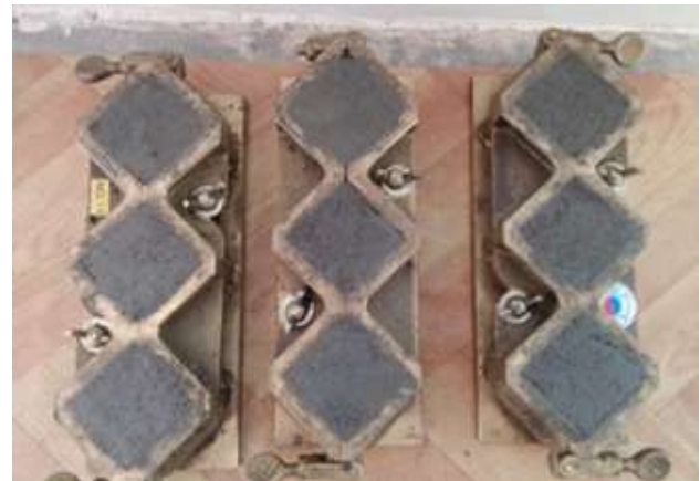
Fig. 4. Specimen for compressive strength of mortar
