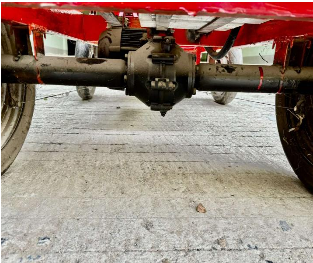
Fig. 2. Installation of motor
