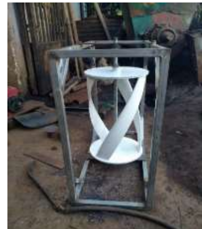
Fig. 6. Turbine and frame constructed
