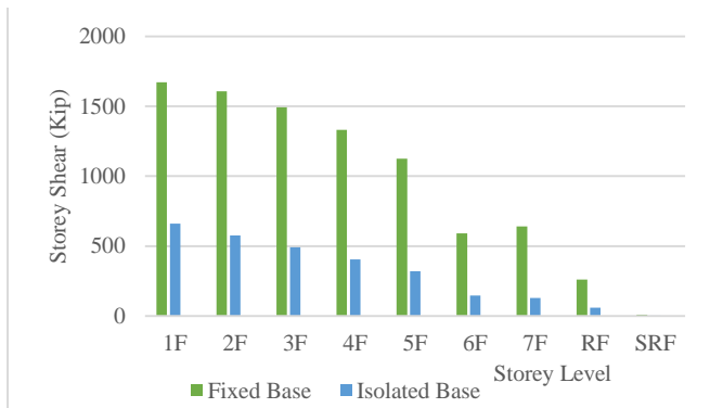
Fig.7. Comparison of storey shear in Y direction.
