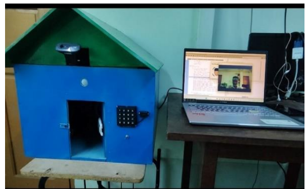
Fig. 12. Operation condition of the door lock system
