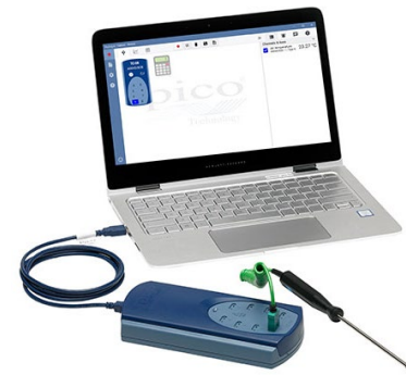
Fig. 10. Pico data logger with PicoLog® software
