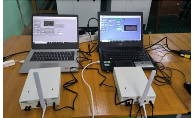
Fig. 4. The hardware setup for two computer and USRP
