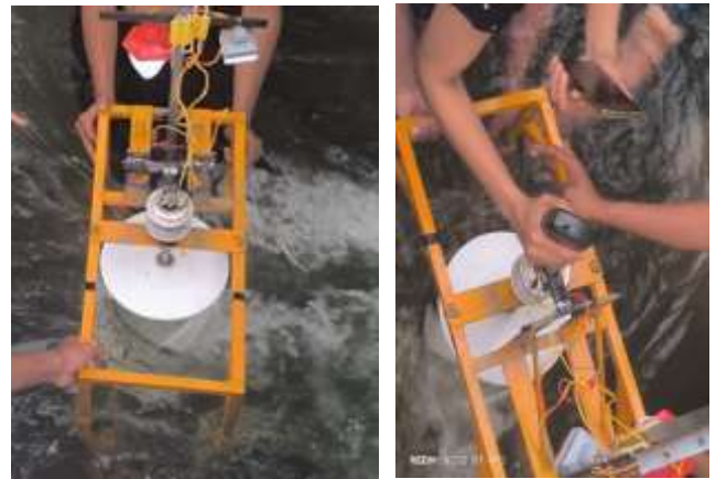
Fig. 10. Performance testing of Gorlov helical turbine
