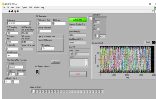
Fig. 19. Front panel of FSK transmitter using IQ sampling rate 100k with samples per symbol 6
