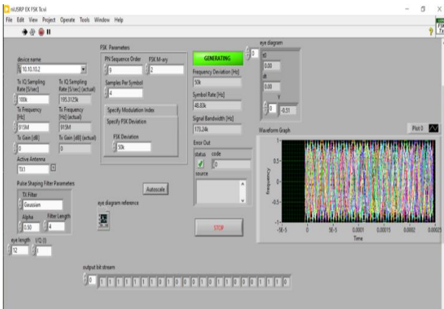
Fig. 13. Front panel of FSK transmitter using IQ sampling rate 100k with samples per symbol 4
