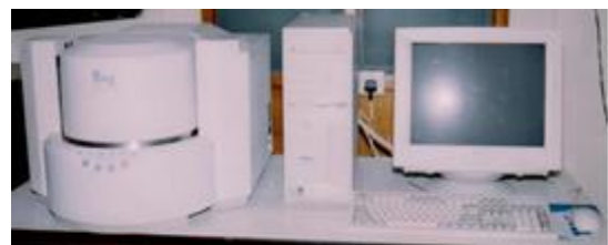
Fig 4. Shimadzu EDX-700 Spectrometer are used to analyze the elements at the University of Yangon's Universities' Research Centre (URC)
